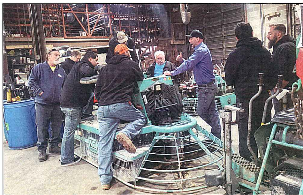
Derek Adams, field service manager of Multiquip, pointed out necessary preventative maintenance needed to use the trowels, including proper greasing, oil changes/hydraulic oil and engine oil.
